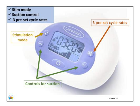
This pump has a stim mode in L upper corner, suction control with the + and – buttons, and the R upper button has 3 preset cycle rates to choose from
