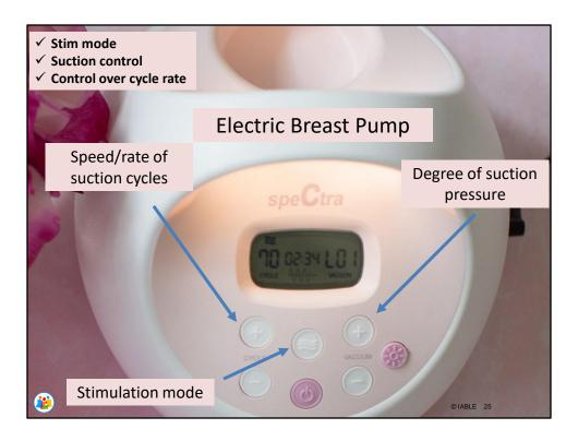
The Spectra breast pump has a stimulation mode, but it does not start on the stimulation mode. When turned on, the pump starts on the expression mode, and the person has to push the stimulation button to start the stimulation mode. It will stay in that mode until the button is pushed again.
